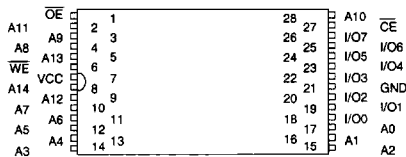
TSOP Top View
